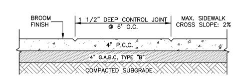
4" PORTLAND CEMENT CONCRETE SIDEWALK DETAIL NOT TO SCALE
