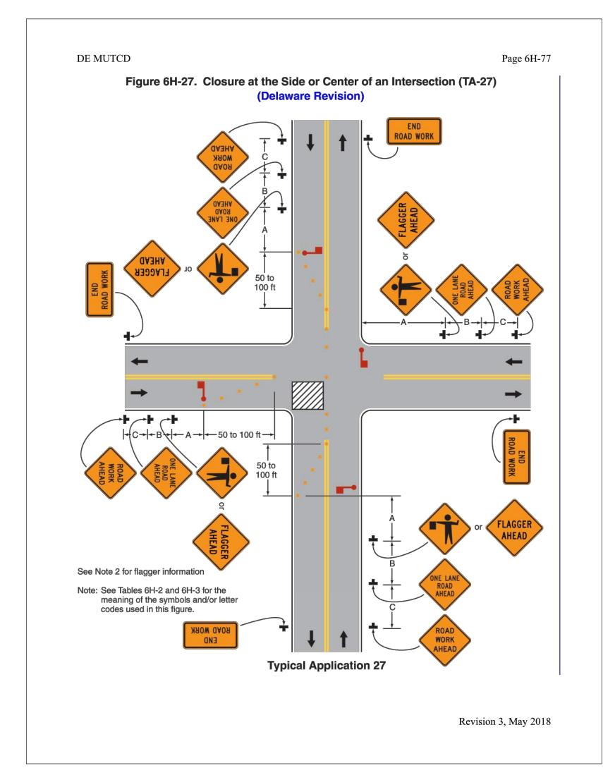
MOT NOTE: USE THIS DETAIL WHEN WORK AND EQUIPMENT IS WITHIN THE ROADWAY AT OR NEAR AN INTERSECTION.
