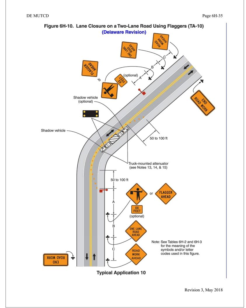
MOT NOTE: USE THIS DETAIL WHEN WORK AND EQUIPMENT IS WITHIN THE ROADWAY.
